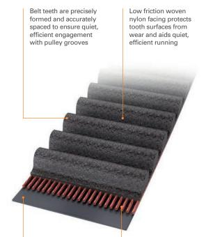
Flexible, durable chloroprene backing polymer encapsulates the tensile cords and protects them from containments and mechanical damage
